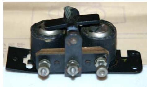
Bruce Kubik found this Madison Hardware M-53 relay, for use with Lionel trains, complete with wiring diagrams and instructions. It could be used to "program" the operation of several trains on the same layout. There aren't any electronics here!
