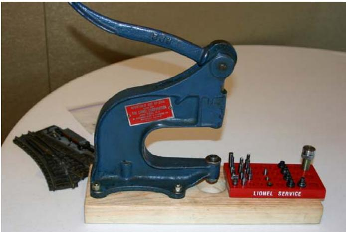
Don Johnson is the owner of this Lionel ST-350 press. This was the essential tool for Lionel Service Stations. The press was used to press drive wheels onto axles, do riveting, and a host of other operations. His press was made 1950-52.
