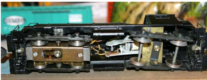
At Left: Mark also brought in this GMC handcar of the 1948-50 era). The gap-ring motor (with the armature attached to one axle) required a push to get started, and there was of course no reverse!
