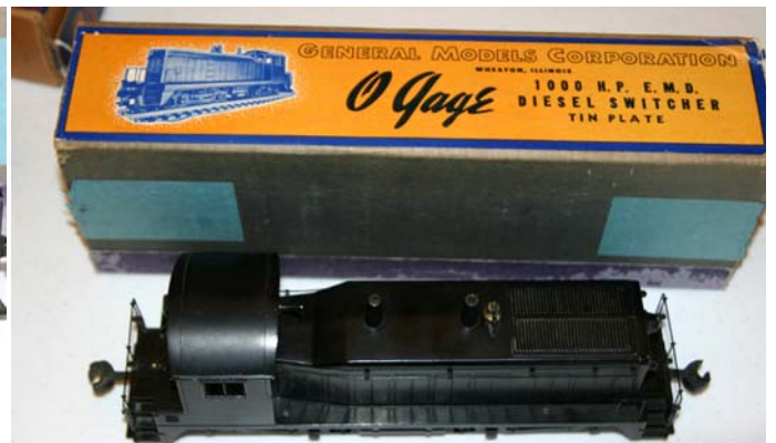
Mark Boyd owns this General Models Corporation EMD diesel switcher (circa 1948-50). As the box indicates, this is a tinplate version, as indicated by the coarse flanges, (dummy) couplers, and reverse unit. But where are the third-rail pickups? This switcher was available as a kit in 2 and 3-rail, and as a ready-to-run, painted version in 3-rail only.
