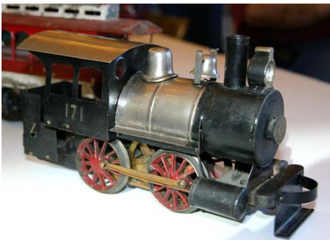
At Right: Chuck Schafer's Carlisle and Fitch #20 "Tank Locomotive," of 1905- 1907. (20 volts, AC or DC). Carlisle and Fitch and Vo.tamp trains are 2-rail, 2-inch gauge.
