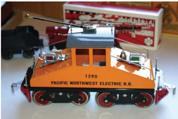
This is Ira Keeler's latest project, an interurban electric locomotive, in Standard Gauge. It is constructed of sheet aluminum, with McCoy trucks, pilots and trim. This is the pilot model for a planned limited production run. This a beautiful, impeccably constructed model. Details of construction are on page 4.
