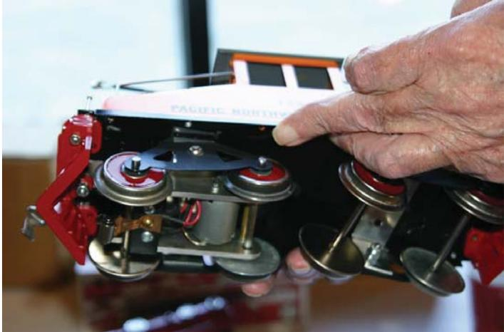
From Page 1: Ira Keeler’s “pilot” model interurban locomotive features a power truck of his own design, shown above and at the right. It incorporates a small motor, obtained from McCoy trains, geared to one axle of the truck. One or two power trucks are possible.
