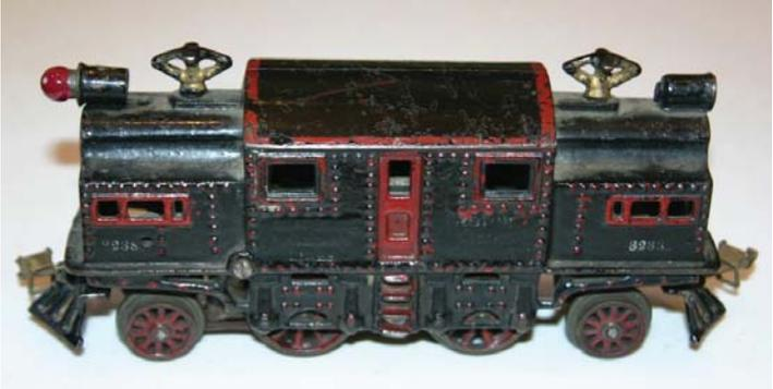
This is Craig Miller's Ives O gauge #3238 loco, from 1914-16 . It has a cast iron body, and a manual reverse. The pilots swivel with each 2-wheel truck.
